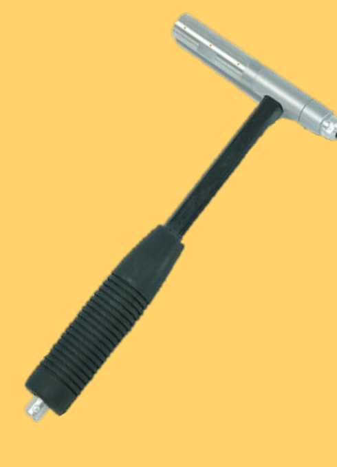
Figure [2b]: Modal Hammer for the experiment
